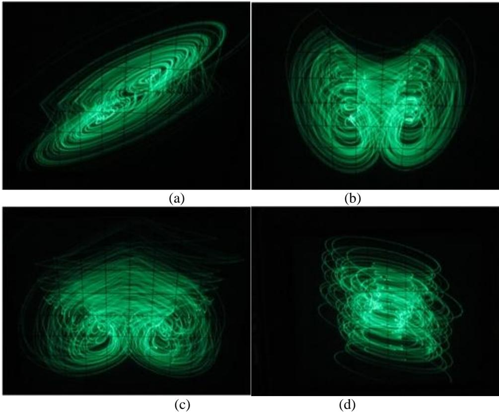
Fig.8 Oscilloscope traces of hyperchaotic attractors of system (3) (a)  $x$ - $y$  plane, (b)  $x$ - $z$  plane, (c)  $y$ - $z$  plane, (d)  $x$ - $u$  plane (1V/div).
