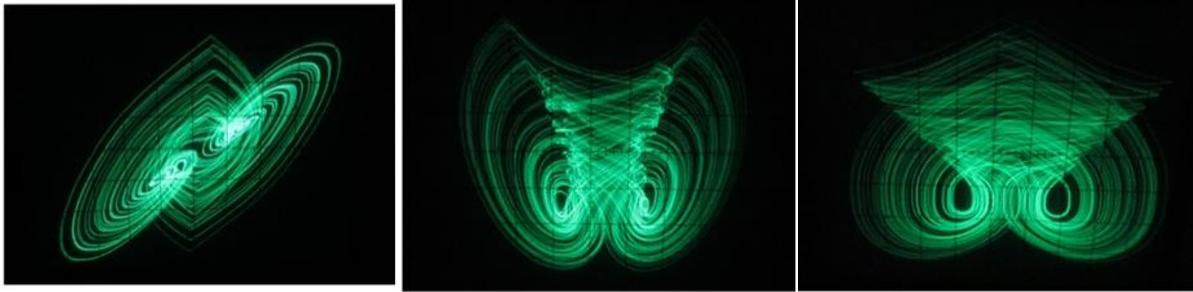
Fig.9 Experimental phase portraits of system (2) (a)  $x$ - $y$  plane, (b)  $x$ - $z$  plane, (c)  $y$ - $z$  plane (1V/div).
