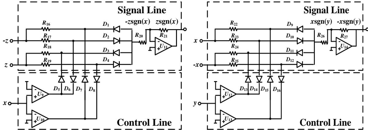
Fig. 6 signal line and control line combined to realize the signum operation
