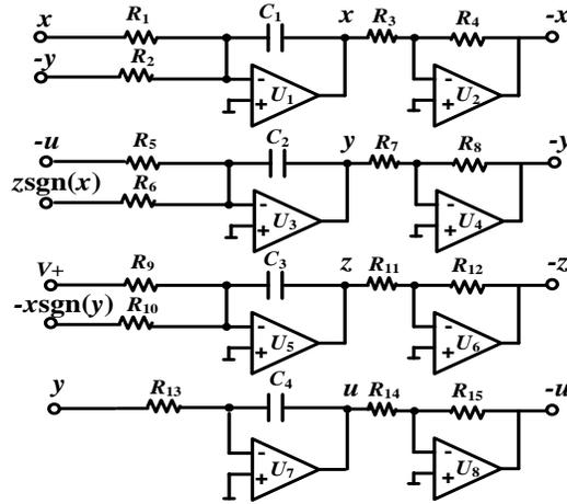
Fig. 7 Four integration channels in circuit structure for the 4-D system (3).
